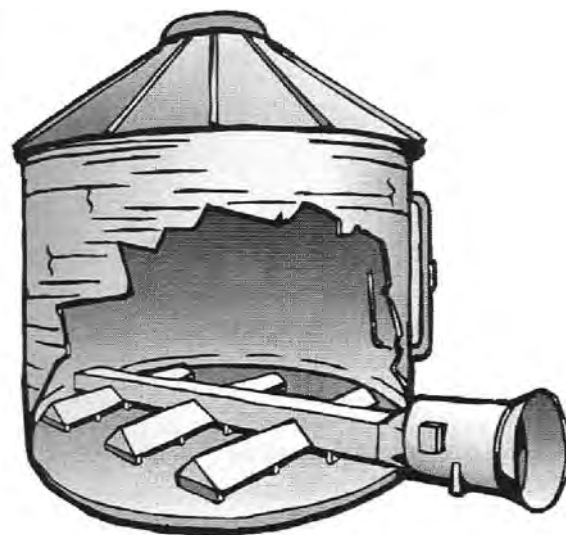
Grain storage recirculation system
